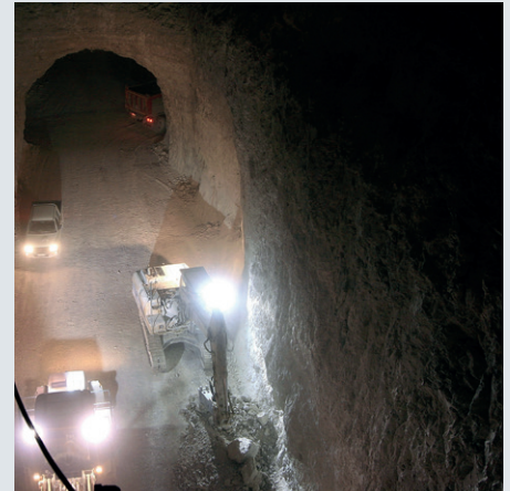
Sector of mine busy with vehicles – Ventsim CONTROL will automatically detect this and adjust airflow accordingly.
